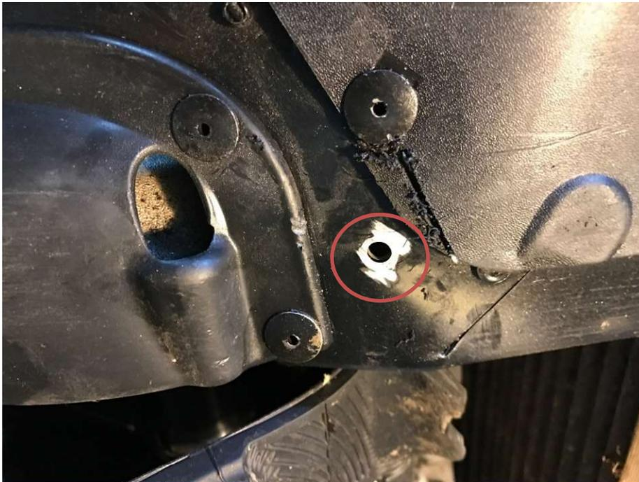
3. (Viper Only) Once plastic is trimmed, attach protector at the hole drilled in step 2. Ensure the inside protector edge is parallel to the inside of tunnel. Drill the second front mounting hole and install a mounting bolt and nut. Nuts go on the inside so bottom is snag free.
