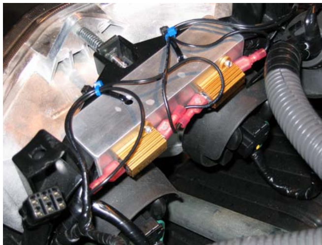
Figure 4, Bracket with resistors mounted.
