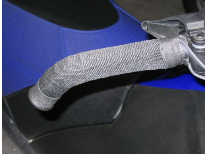
Figure 3, With fabric heat shrink in place.
