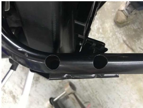
6. Install the grill. Use the (2) oem torx screws you saved in step 1 for the top two mounts and a 25mm long bolt provided for the lower mount.
