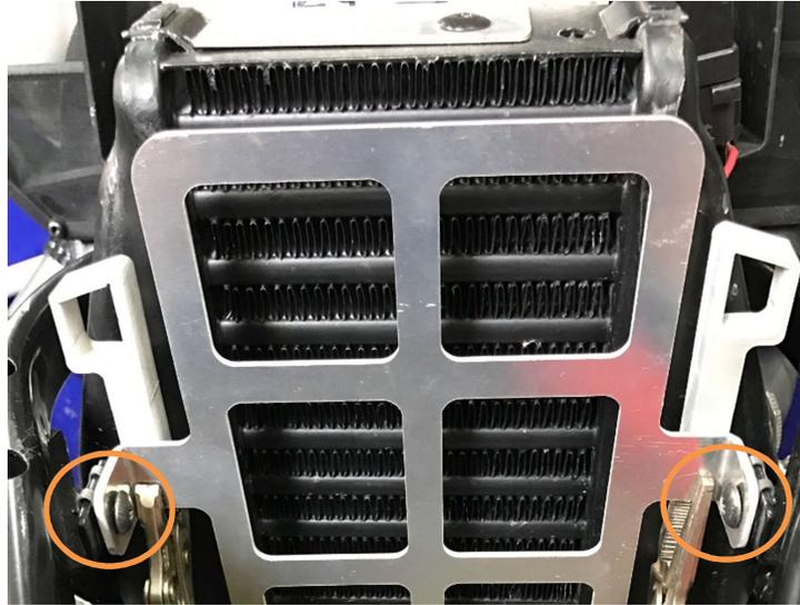
7. Once the nose skid plate and grill are secured, tighten (4) bumper bolts back up.
