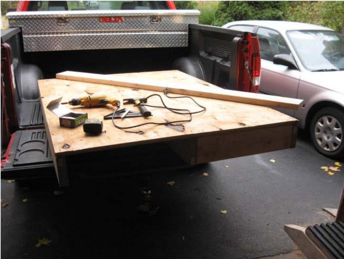
I used turnbuckles in the corners to attach it to the bed. The turnbuckle came with 1 hook and 1 eye, I sawed a little off the eye to create 2 hooks. I mounted the screw eye slightly higher and away from the bed hook. When tightened it pulls the deck down and towards the cab.
