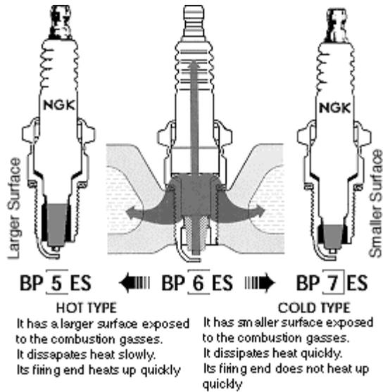
The insulator nose length is the distance from the firing tip of the insulator to the point where insulator meets the metal shell. Since the insulator tip is the hottest part of the spark plug, the tip temperature is a primary factor in pre-ignition and fouling.
