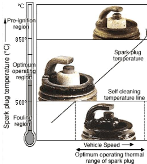
The firing end appearance also depends on the spark plug tip temperature. There are three basic diagnostic criteria for spark plugs: good, fouled and overheated. The borderline between the fouling and optimum operating regions (500°C) is called the spark plug self-cleaning temperature. The temperature at this point is where the accumulated carbon and combustion deposits are burned off.
