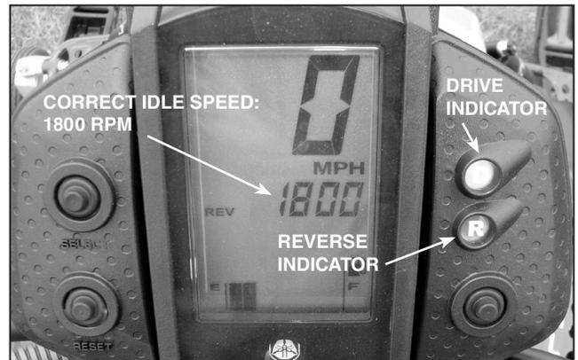
**Remedy:** Confirm correct idle speed, TPS function, and shift operation as instructed in this bulletin. If the unit still has a shifting problem, install an additional shim and a new-style drive belt per bulletin instructions (this new belt is standard on 2009 and later models).
