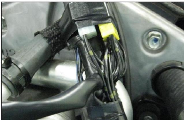
13. Route the new wire sub-harness using the four existing cable ties, as illustrated.
